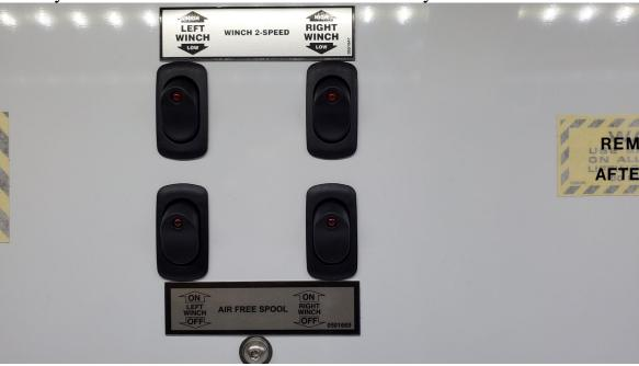
Note: labels should be installed after the assembly of the control station is complete. Vulcan LH Control Station (with Third Winch Option shown)
